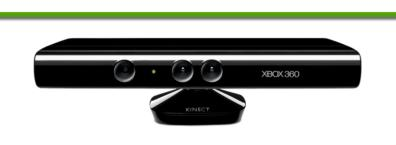
Using the infrared (IR) camera, Kinect can recognize up to six users in the field of view of the sensor. Of these, up to two users can be tracked in detail. An application can locate the joints of the tracked users in space and track their movements over timé.
